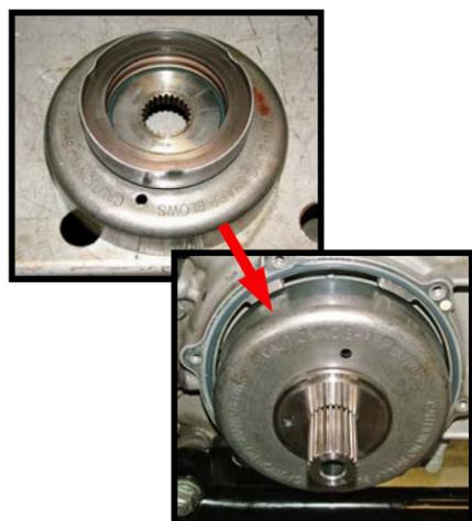
The stock rotor needs to have the compensator assembly machined off to be used with this kit. Tech Cycle can provide you with a modified rotor or machine your stock unit to fit.
