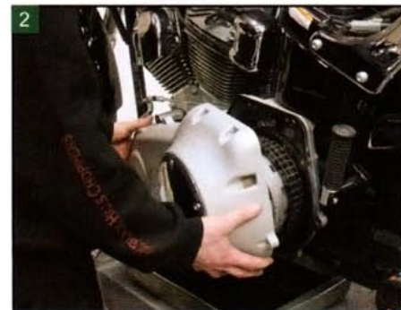
2 Once the primary fluid has been drained, carefully remove the outer primary cover.
