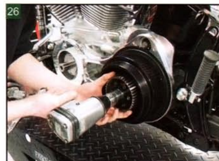
Use an impact wrench to install the clutch hub retaining nut.
