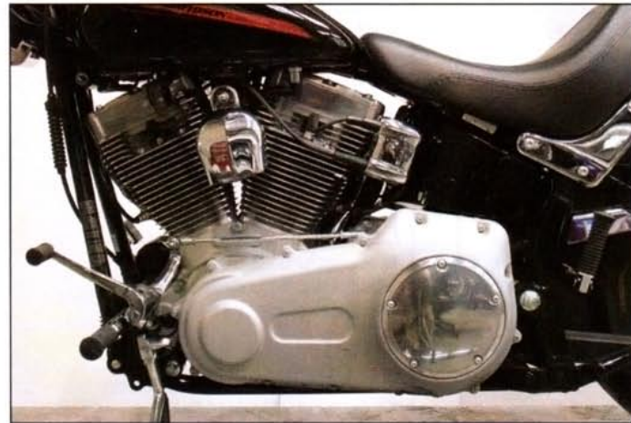
Here is the factory primary assembly on our shop '07 Softail Standard.
