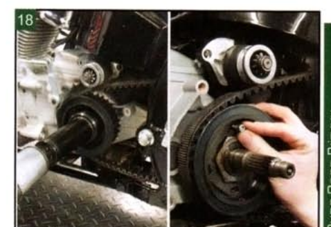
18 Use an impact wrench to install the locknut and then install the locknut lock plate and tighten the bolts.
