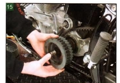
15 Then remove the factory belt sprocket from the transmission mainshaft.
