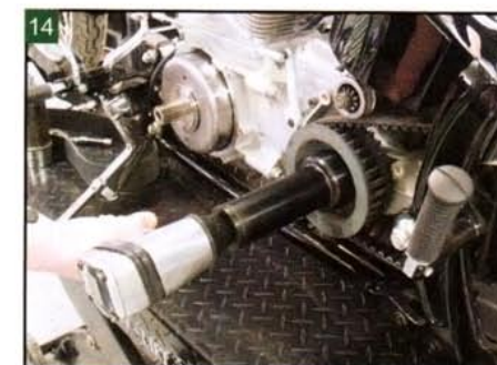
14 Remove the lock nut. NOTE: On the '07 Softail this nut has left hand threads as opposed to older models.
