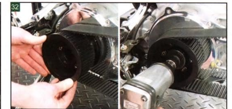
Place the primary belt over the rear pulley and slide the front pulley through the belt and onto the mainshaft. Secure the front pulley with the factory bolt.
