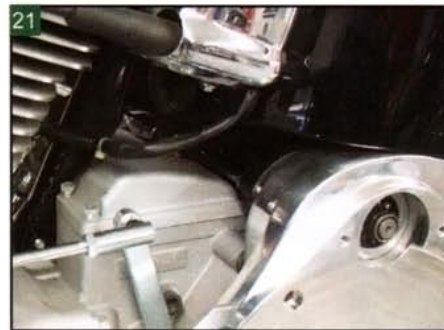
Install the starter into the backside plate and tighten the two starter mounting bolts.
