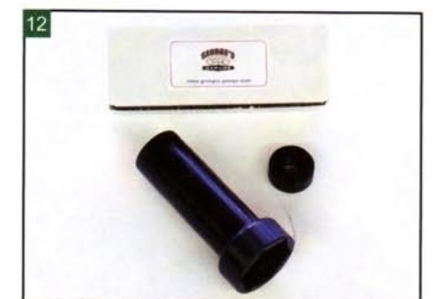
12 This is the second George's Garage tool we used; this tool removes the transmission mainshaft lock nut.
