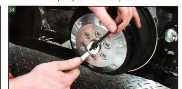
Collapse the clutch cable adjuster and adjust the clutch by turning the set screw until it touches the transmission push rod, then back off 1/2 turn and set the locking nut.
