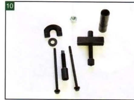
10 This is the George's Garage specialty tool used to remove the race from the transmission mainshaft.
