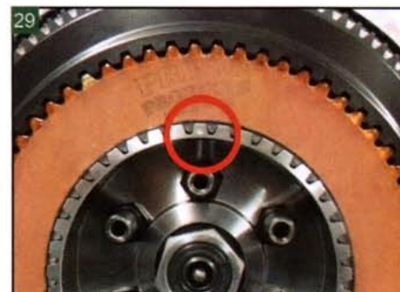
This is the dot on the clutch basket.
