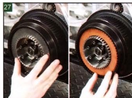
Install the clutch plates starting with the thickest metal one, then alternating fiber and steel plates.
