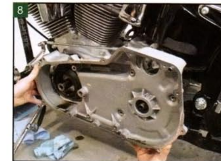
8 Now remove the inner primary from the engine and transmission cases.
