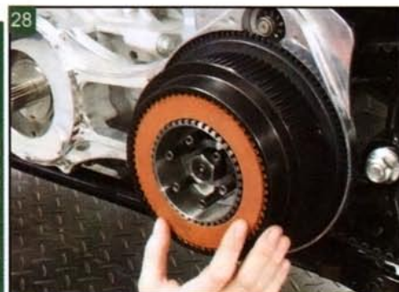
The last plate to be installed is a fiber friction plate.
